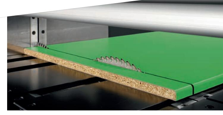
PFS function, avilable on Selco WN 250 machine, for making cuts on soft and post-formed panels. A special NC program that ensures the perfect finish of both the entrance point and the exit profile, preventing any splintering of fragile, delicate materials (patented).
