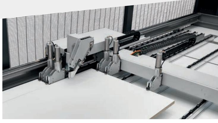
The Twin Pusher system offers an additional pushing device consisting of two fixed collets. It permits simultaneous cutting, which drastically reduces the cycle time.
