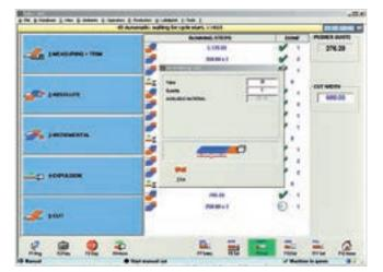
Interactive program for the quick, easy execution of cuts and grooves, even on recycled panels.
