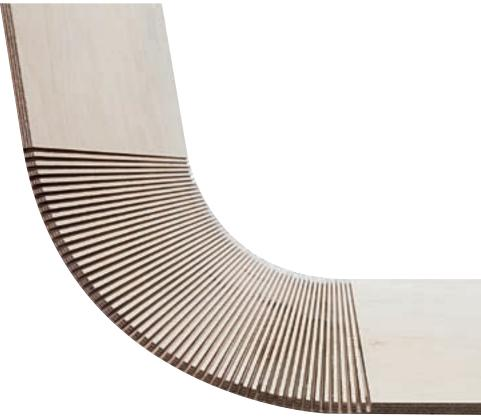
System for the automatic execution of grooves, the width of which can be programmed via the numerical control. The groove depth can be adjusted manually from the outside of the machine and with the blades moving.
